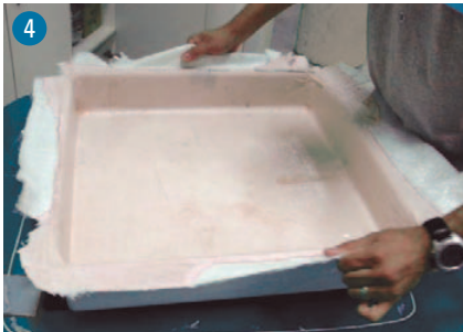
4 Demold after resin cures
